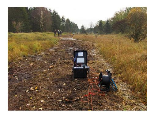
Figure 6.5: Electrical resistivity surveying.
