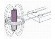
Figure 12.6: Faraday showed that, by moving a magnet in and out of a coil of wire, he could generate a current in the wire.
