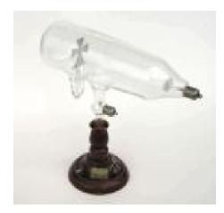
Figure 13.1: The discovery that gasses at low pressure can conduct electricity led to a series of remarkable discoveries. Here we see a "Crookes tube" used by Sir William Crookes to repeat and refine the early work of Plücker and Geisler.
