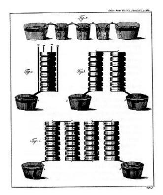
Figure 12.4: To prove his point, Volta constructed the first electrical battery. In the figure, we see his first battery and some Voltaic piles.
